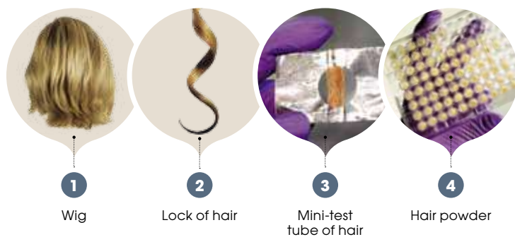
Miniaturising the tests means that now only a few milligrams of hair powder can be used to test hair products.
